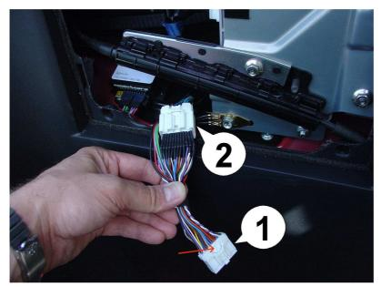
3. For better visualization the locking mechanism is shown on the smartTOP plug (1), marked with an arrow. It needs to be pushed down while pulling hard on the plug. Once the plug is out, plug it into the matching socket on the smartTOP wiring harness (2).
