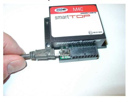
This module comes with our USB Field Upgrade and Configuration Port! BEFORE YOU INSTALL, we encourage you to connect the module using the supplied USB cable and check for firmware updates. All information and software regarding this new feature can be found at
