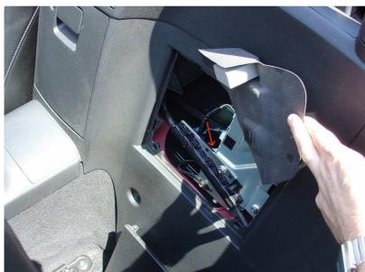
2. Lift up the padding to reveal the convertibe top controller. The bottom plug (marked with the arrow) will have to be removed in the next step.
