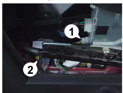
4. Connect the smartTOP plug (1) to the top controller, then connect the smartTOP module to the harness. Turn the ignition on. A rapidly blinking green LED (2) will indicate proper installation. Lastly, program the module as desired, according to the operation manual.
