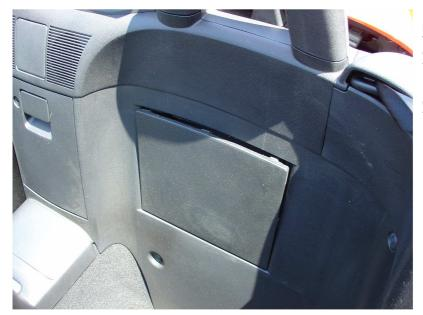
1. Open the convertible top for better access. IMPORTANT: Turn off ignition and pull key out before continuing! Open the cover behind the driver's seat (left side of the car) as shown. Use a flat screw driver or any flat object like a coin to pry it out on the top.
