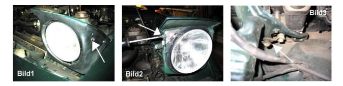
Pull the plug off the back of the headlamp.
