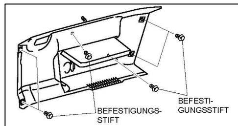
For the side trims. Remove all the fasteners as show below, and remove the two trims.
