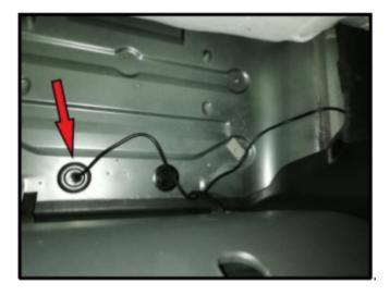
7. Pull the plug about 60 cm, make sure that the cable is behind the heat shield.
