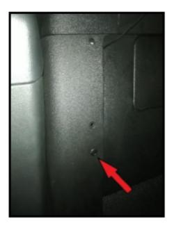
9. Pull the power cord into the 12V cigarette lighter socket the socket is hidden under the passenger side foot.
