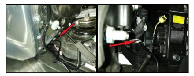
10. Pull the cable behind the passenger backrest and the central console. Plug the plug into the cigarette lighter socket, which is located under the dashboard in the passenger foot well.
