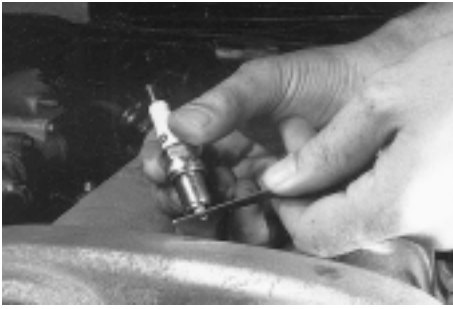
6/6 Measuring sparkplug electrode gap.
