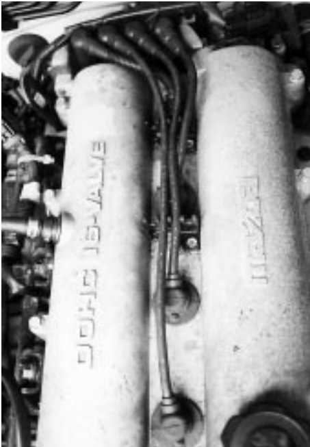
6/7 Correct connection of sparkplug wires.
