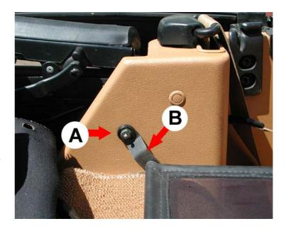
attach the end clip but only turn it once so its just resting on there, holding the bracket in
